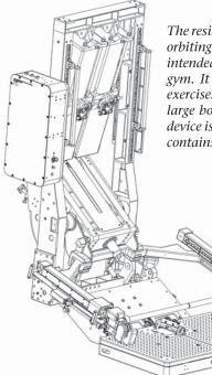
The resistive exerciser used by astronauts on the orbiting space station is a full body exerciser, intended to simulate free weights, like a home gym. It lets them perform cable and bar-type exercises for a single hand, leg, or limb. The large box on the upper left side of the exercise device is the ARED Instrumentation Box, which contains the four IOtech Personal Daqs.
