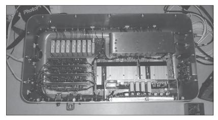
The four pairs of circuit boards in the lower left corner of the box are four Personal Daqs with cases removed and connectors replaced with direct solder connections. This is the first build of the actual hardware that is used for simulation and actual flight.
